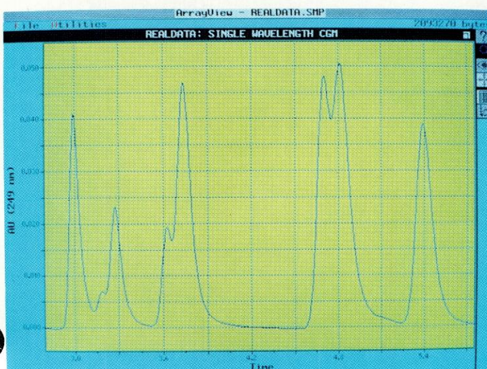
Chromatograms can be viewed at any wavelength for selection of optimal settings.
