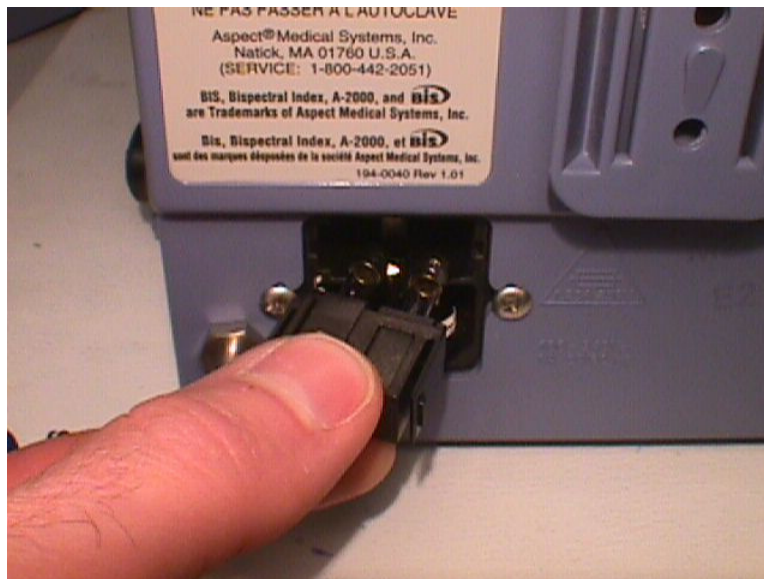
Figure 7-23 Re-installing the fuse holder
