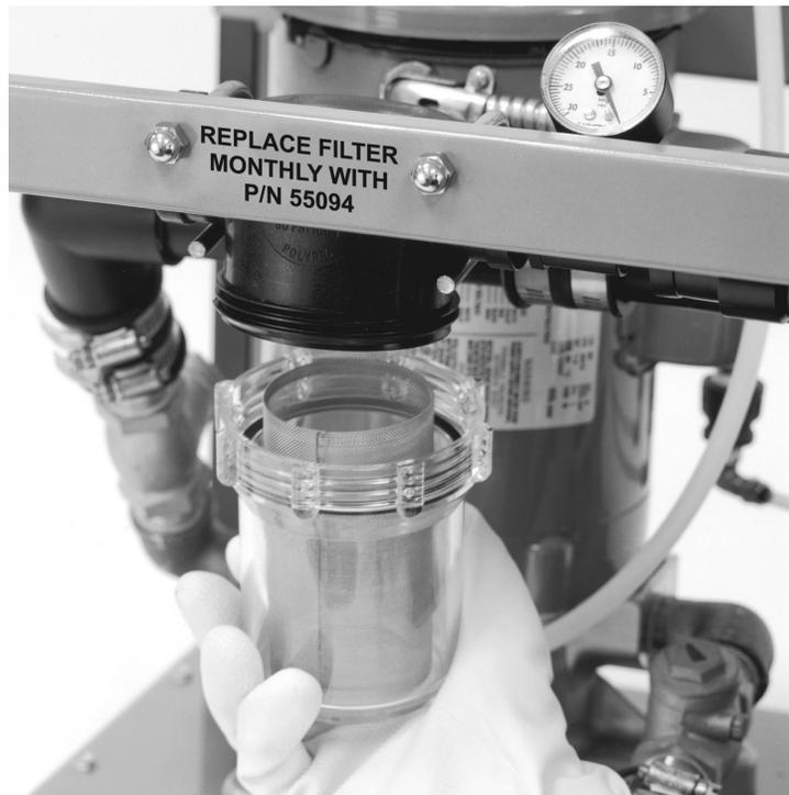
Figure 12. Intake Solids Collector Location
