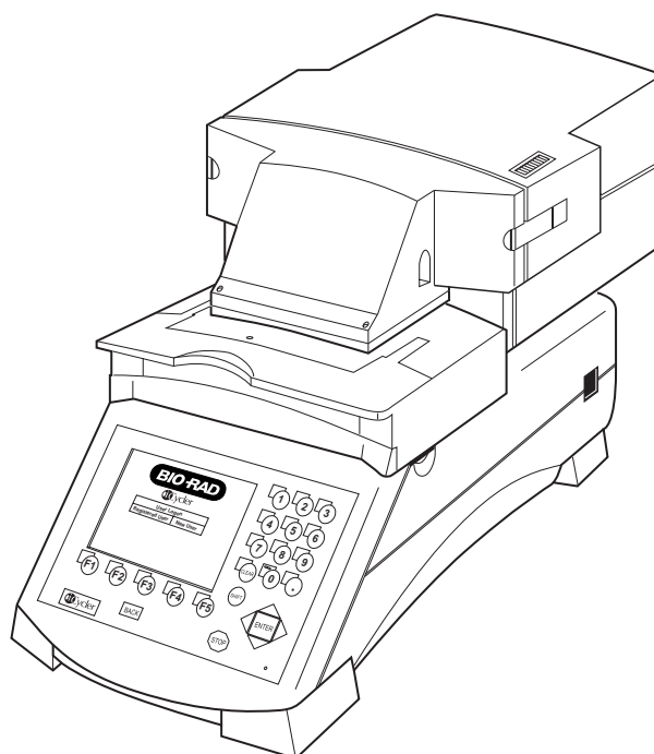
Fig. 1.1. Optical Module Upgrade to iCycler Thermal Cycler.
