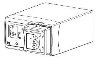
**3.** Turn on power to the smoke evacuator by pressing the on switch ( I ) located on the front panel.
