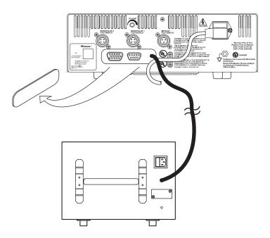
**7.** *(Optional)* Connect the RapidVac Footswitch to the front panel of the smoke evacuator. Use only Valleylab footswitches with the RapidVac Smoke Evacuator.
