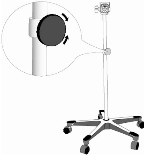
Figure 13. Adjusting the height of the mobile stand.
