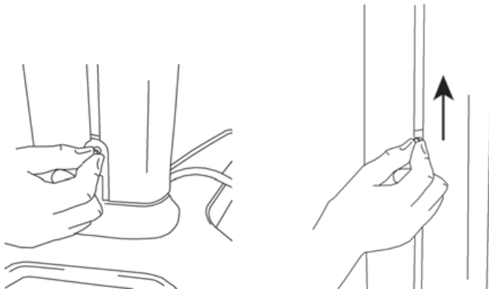
Figure 3 Inserting the nut plate into the groove at the back of the column and sliding it up the column
