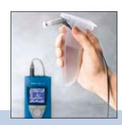
Ergonomic screening handle You can use the optional handle detached as illustrated or with the handle mounted on the OTOflex.
