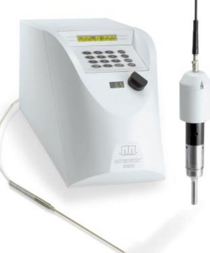
Over-heating a sample is no longer a worry now that the Sonicator® 3000 has the capability of temperature control. The sample is monitored by a temperature probe and when the pre-set temperature of your sample is exceeded, an external cooling device can be triggered ensuring your sample remains within your desired temperature range.
