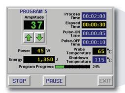
This screen is an example of a program in progress. Amplitude, pulse on/off time, temperature and energy delivered values are all clearly displayed.
