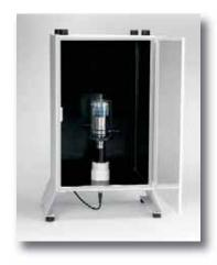
The Sound Enclosure (#432B) is highly recommended for all Cup Horn users. In addition to reducing sonication noise to safe levels, it securely supports the Cup Horn in the proper position. The Sound Enclosure features ports on either side to allow coolant tubing to pass from the Cup Horn to a water source or pump system outside the box.
