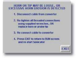
The Sonicator's fault detection circuitry has detected a failure. A self diagnostic test will identify the problem and give instructions on how to clear the error.
