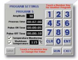
This Program Setting screen enables the user to set the parameters for their program. Up to 10 individual programs can be saved.
