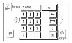
If you want to weigh up to a target value, press the "**Nominal**" function key, and specify the target weight for the first component.
