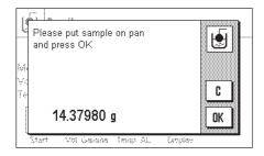
Press the "**Start**" function key to start the density determination. You will then be prompted to place the sample on the pan (without the gamma sphere).
