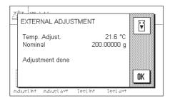
The balance confirms successful completion of the adjustment. Press "OK" to return to the application.
