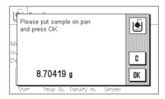
Press the "Start" function key to start the density determination. The balance will automatically carry out a taring, after which you will be prompted to put the solid body in place (weighing in air).
