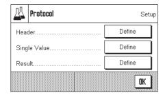
You can make the settings for the printout, divided into header, individual values and result, in the three submenus. Additional settings, described below, are available for Formulation.
