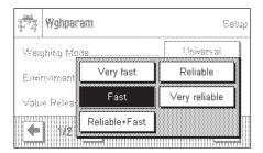
With this setting you can specify how rapidly the balance considers the measurement to be stable and therefore releases the value. The "Very fast" setting is recommended if you require rapid measurements whose repeatability is of lower significance. The "Very reliable" setting gives measurements that are highly repeatable, but it lengthens the stabilization time. Three other intermediate settings can be selected.
