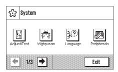
**Change system settings:** If you want to change system settings that apply to the entire weighing system, i.e. to all the applications, then press the "...." key and then the "**System**" button. The system settings are described in detail in Section 5.
