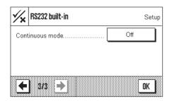
If under "Host" the built-in RS232C interface has been selected, you can additionally activate **Continuous mode**.
