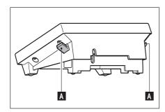
For a steeper reading angle, pull both levers (A) at the side upward. You can then pull the upper part of the terminal slowly upward until it engages in the desired position. Three different setting positions are provided.
