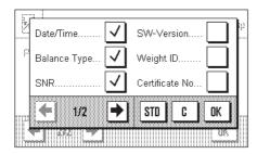
In this menu, which covers two pages, you can specify the information to be printed on the adjustment and test records.
