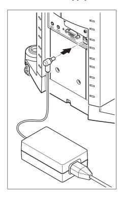
Your balance is delivered complete with an AC adapter and a country-specific power supply cable. The AC adapter is suitable for all power supply voltages in the range:  $100 - 240 \,\text{VAC}$ , -10/+15%,  $50/60 \,\text{Hz}$ .
