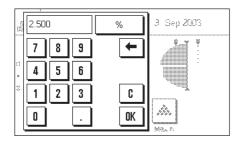
You can use the two "+Tol" and "-Tol" function keys to specify the precision to be used for the weighing. The input window is the same as that for the target value. Both tolerances are set at the factory to 2.5%.
