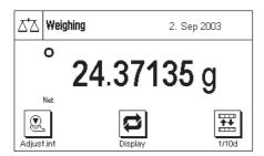
**Weighing:** Open the glass draft shield, insert the items to be weighed, and close the glass draft shield again. As soon as the stability detector icon (the small circle to the left of the weight display) goes out, the display is stable and you can read off the weighing result. The stability detector icon is still visible in this diagram, and therefore the weighing result is not stable.
