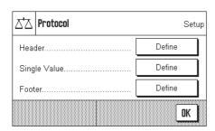
For the sake of clarity, this large menu is divided into three submenus in which you can specify the options for the printout header, the printing of the individual values, and for the footer.
