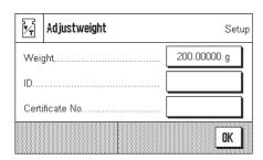
If you work with an external adjustment weight, you can specify its properties here (**Note:** In accordance with country-specific regulations, this function may not be available on certified balances).
