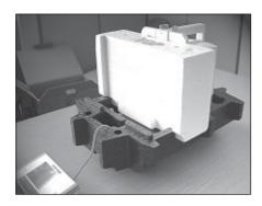
Insert the packing set with the draft-shield glass into the packing cushion (see illustration).
