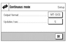
In "Continuous mode" you can specify various different data formats (MT–SICS, PM, AT, MT) depending on which peripheral device is connected. You can also specify the update rate per second (2, 5, 6, 10).
