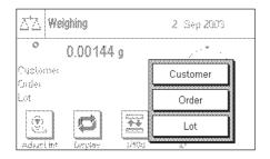
If you want to carry out an order for a customer in the application, press the "ID" function key. You can then select the identifier for which you want to enter text (e.g. "Customer").
