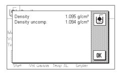
The balance now determines the density of the paste, and then displays the result (the compensated and/or uncompensated value, depending on the settings that you have made for output of the result, see Section 9.3.5).
