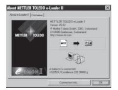
Before you update the software of your balance, please check in the "Help" menu that the communication with the balance is functioning. (In the example shown here, the e-Loader II is confirming that a balance is connected.)
