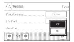
"**Off**": The weighing result is not automatically printed out, and the "\(\begin{align\*}=\)"
