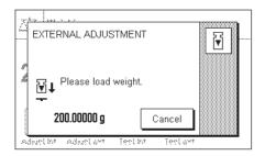
If there is a weight on the weighing pan at the time of the adjustment, the flashing display "0.00000g" prompts you to remove it. You will then be prompted to place the adjustment weight on the pan. The required adjustment weight is indicated at the lower edge of the window.
