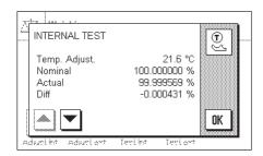
Successful completion of the checking process is confirmed with the window shown here. If a printer is connected to the balance the check will automatically be recorded on a hard copy in accordance with the specifications that you have made for printing out checks in the system settings (Section 5.3.4). You will find a sample printout in Section 6.4.6.
