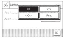
Select the desired function for each switch: "Print", zero setting (" $\rightarrow 0 \leftarrow$ ") or taring (" $\rightarrow T \leftarrow$ "). If no switch is connected to the corresponding Aux connection, or if you want to deactivate it, select "Off".
