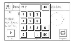
If you are using **water or ethanol as the auxiliary liquid**, enter its **temperature** using the "**Temp. AL**" function key. (Density tables for these two substances covering the temperature range from  $10^{\circ}\text{C}$  up to  $30^{\circ}\text{C}$  are stored in the balance; see also Sections 9.7 and 9.8.). The illustration here shows the corresponding input field (input in  $^{\circ}\text{C}$  with 1 decimal figure).
