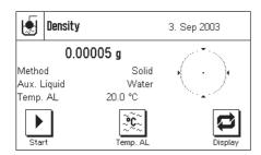
In the application-specific settings, select "**Solid**" as the method (Section 9.3.2) and specify the auxiliary liquid that will be used (Section 9.3.3).
