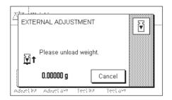
At the end of the adjustment procedure, you are prompted to lift off the weight. Remove the adjustment weight from the weighing pan.
