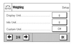
"Display Unit": Specifies the unit in which the result will be displayed
