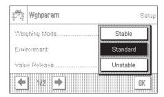
With this setting the balance can be ideally adjusted to match the ambient conditions at its location. If you are working in an environment which is practically free from drafts and vibrations, choose the "Stable" setting. If, on the other hand, you work in an environment where the conditions are continuously changing, select "Unstable". The "Standard" setting corresponds to an average working environment subject to moderate variations in the ambient conditions.
