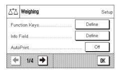
**Change application-specific settings:** If you want to change the settings for the active application, press the "=:" key. Information on the application-dependent settings can be found in the description of each individual application (Section 6ff).
