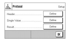
Additional settings for statistics, described below, are available in the three submenus in which you can specify the options for the printout header, for printing the individual values, and for the result.
