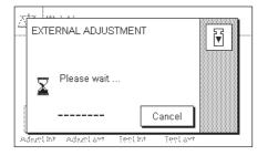
The adjustment process continues automatically once the required weight has been placed on the pan. The window shown here is displayed during the adjustment.
