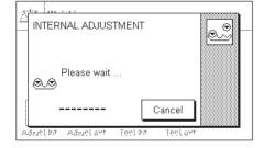
Pressing this function key triggers an adjustment of the balance using the built-in adjustment weight. You can do this at any time; you can also specify in the system settings that the balance requests adjustment as soon as a specified change in ambient temperature has taken place ("CalInfo" setting, Section 5.3.1).
