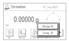
Press the "ID" function key and enter the desired names (for the formula, for the first component and, if ID3 is active, also for the current lot).
