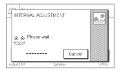
As soon as the specified temperature criterion is satisfied, the small FACT icon appears in the top right-hand corner of the display. The balance indicates in this way that it wants to carry out a FACT adjustment. Note: during the first 24 hours following connection to the mains, FACT will execute a number of times, regardless of what criterion has been selected.
