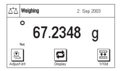
The factory setting of the balance displays the weighing result at a size so that it can easily be read. In this display mode neither the information fields nor the graphical "SmartTrac" filling guide are visible.
