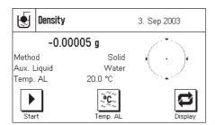
The following display appears when the application has been selected. Special function keys and information fields for density are activated under the factory settings. The balance is preset to determine the density of solid objects using water as the auxiliary liquid. You can adapt these settings to your own requirements, as described in the following Sections.
