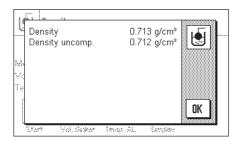
The balance now determines the density of the liquid, and then displays the result (the compensated and/or uncompensated value, depending on the settings that you have made for output of the result, see Section 9.3.5).
