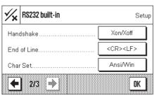
If you have activated a device you can adjust the interface parameters for communication with that device with the "Define" button (baud rate, bit/parity, stop bits, Handshake, end of line, character set, and continuous mode). The parameters are preset to match the corresponding optional devices from METTLER TOLEDO.
