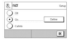
You can make the settings for fully automatic adjustment using the internal adjustment weight in this menu (FACT). FACT (**F**ully **A**utomatic **C**alibration **T**echnology) calibrates the balance under full automatic control on the basis of a pre-selected temperature criterion.
