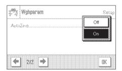
Automatic zero setting ("AutoZero") continuously corrects possible variations in the zero point that might be caused by small amounts of contamination on the weighing pan. You can use this menu option to switch the automatic zero setting on or off.
