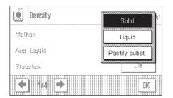
**"Solid":** Determination of the density of non-porous solid bodies with the
