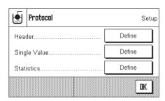
Additional settings for density determination, described below, are available in the three submenus in which you can specify the options for the printout header, for printing the individual values, and for the statistical printout.
