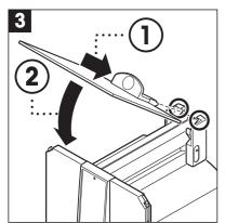
Insert the top door of the draft shield at an angle (slightly less than 30 degrees) into the guide positioned at the back, and swivel the draft-shield door carefully down.
