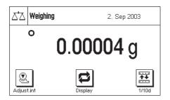
**Switch on the balance:** Switch the balance on by briefly pressing the "**On/Off**" key. Immediately after being switched on, the balance runs the most recently used application.
