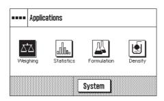
**Select the application:** If you do not want to work with the current application, use the "...." to select the application menu (or alternatively by touching the appropriate zone in the upper left-hand corner of the display). Touch the icon for the desired application, and the relevant software will load.
