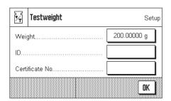
If you use an external weight to check the calibration, you can enter its properties (weight, ID and certificate number) here.
