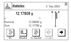
As soon as you have entered the target value and the tolerances the graphical filling guide ("SmartTrac") appears. This displays tolerance marks that make it easier for you to weigh up to the target value: You can add roughly the right amount of material until the lower tolerance value has been reached, and then, if necessary, make careful additions to reach the target value.
