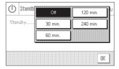
You can switch the energy saving function off ("Off"), or you can specify a period of 30, 60, 120 or 240 minutes after which the balance switches itself into standby mode. The standby mode is the same state into which the balance enters when switched off with the "**On/Off**" key. The "**On/Off**" must be pressed to turn the balance on again.
