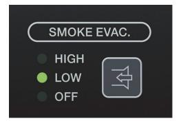
When used in combination with the Olympus MAJ-1939 foot switch, pressing the appropriate switch allows this instrument to execute insufflation into and suction from the cavity simultaneously to exhaust and remove the generated smoke and mist while maintaining the cavity pressure constant. The flow can be adjusted using the toggle button.
