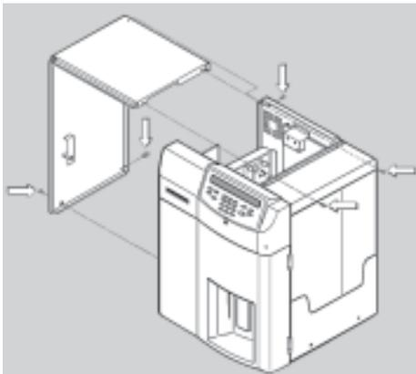
Unscrew the 5 cover fixation screws and remove the cover : pull it backward and lift it up to the rear of the instrument (Diag.9.3).
