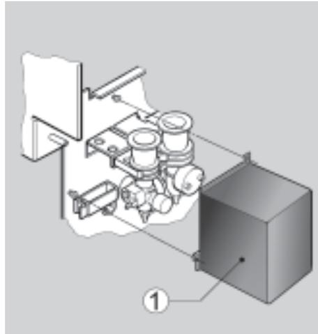
Unscrew slightly the 2 screws of the WBC/HGB chamber protection cover. Remove the cover and check that the chamber is fixed properly in its clips and the electrode block is attached firmly to the chamber (Diag.9.6).
