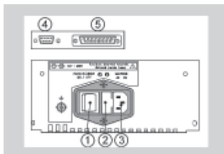
Remove the fuse holder from its location on the rear panel pressing on the holder lock (Diag.9.8) and check the fuse characteristics : they should be 1 Amperes, 250 Volts Slow-Blow.
