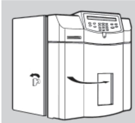
Using the key from the installation kit, unloosen the locker as shown on the Diag.9.2 below. Open the pneumatic protection door.
