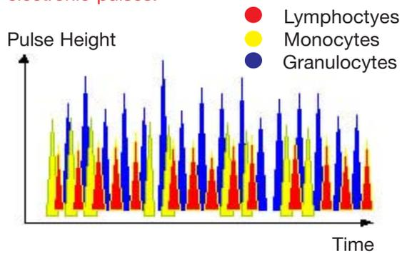
Pulses are grouped according to the Number of cells and the Size of the cells.
