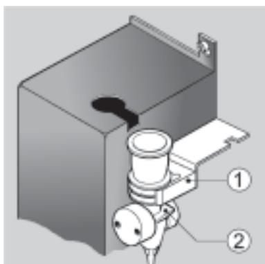
Check the position of the chambers as shown in Diag.9.5. below. Each chamber should be in its proper position with its clips and the electrode block is attached firmly to the RBC chamber.
