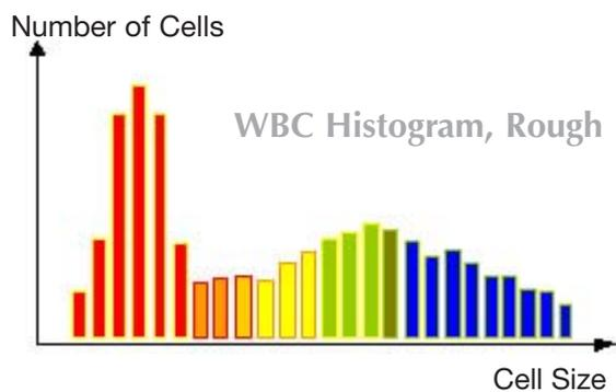
Pulses are electronically calculated and smoothed to show the WBC Distribution curve.
