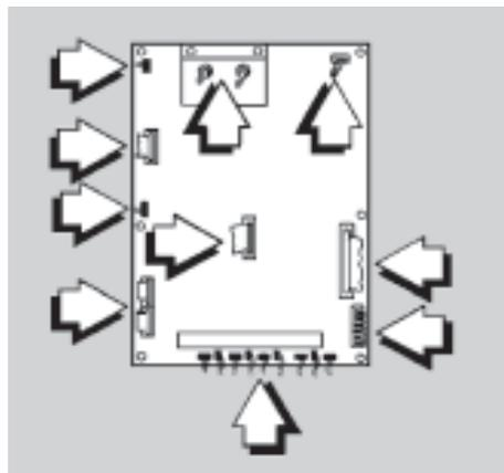
Check that the connectors on the printed circuit board are securely in place (Diag.9.7). Re-install the instrument cover.
