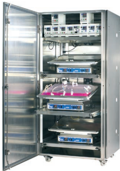
Fig 5. The cabinet fits through standard doorways and it is mounted on casters for mobility. It can accommodate up to four 19" instrument racks on the top shelf and up to three BASE20/50EH series bioreactors on slide-out shelves. In addition, the cabinet has CO 2 /O 2 manifold for gas distribution, removable stainless-steel door and sides.
