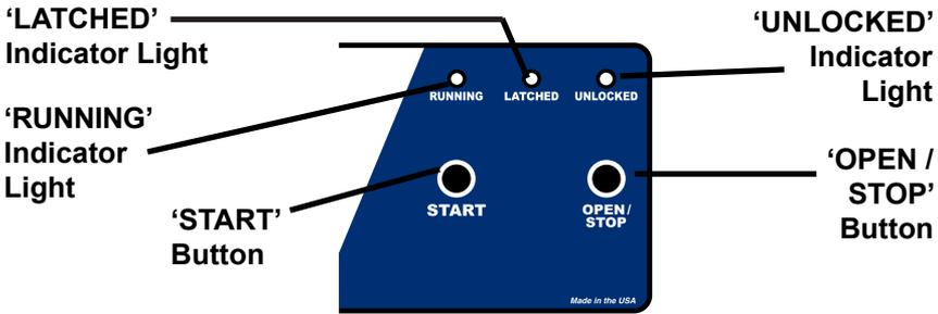
'RUNNING' Lights up when the machine is in operation, (power is being applied to the motor).
