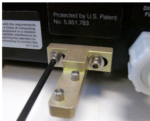
Figure 2: Mount the shipping bracket on the back panel, on the studs provided next to the Fluid In port.
