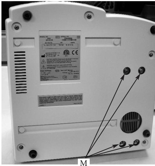
11. Reposition the base assembly upright and reconnect all cable assemblies by reversing steps 7 and 8.
