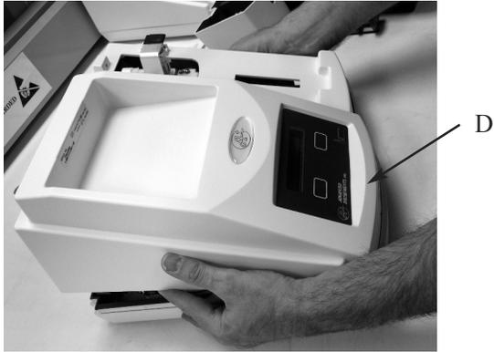
**Note:** Use caution when separating the top and bottom covers to avoid damaging the display and keypad cable connections.
