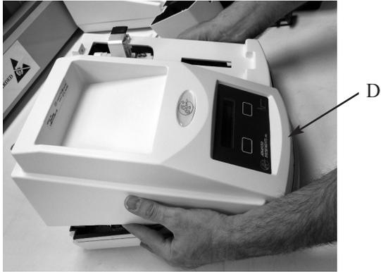
5. Return the instrument to its upright position and carefully rotate the rear of the cover up and away from the bottom cover while keeping the front portion close to the bottom cover (D).
