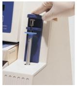
Operating the Advanced Micro-Osmometer Model 3300 is fast and easy. Once the sample has been aspirated into the sample tube, simply insert the tube into the instrument's vertical holder. Push the holder down and testing begins automatically. Results are displayed in 60 seconds.
