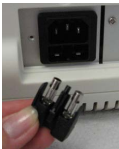
Figure 8.2 NICOM fuses drawer and fuses
