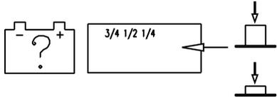
Located on the Smart Pack batteries, a set of four (4) LEDs used to indicate the approximate amount of charge remaining in the battery pack. See Page 107, CHECKING BATTERY STATUS for more information.
