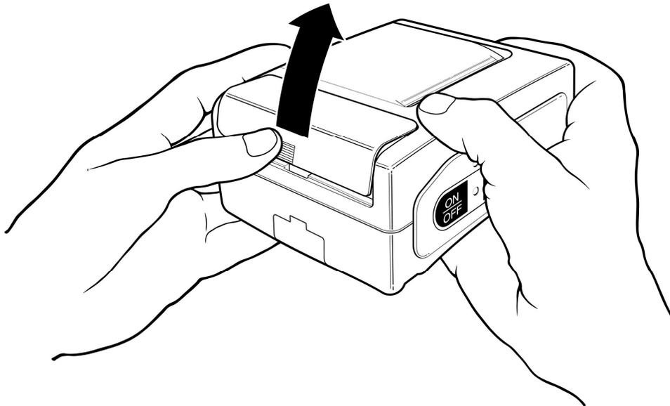
Figure 23: **Opening the Battery Door**
