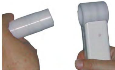
2. Unscrew the mouthpiece counter clockwise, discard the filter and dispose in the clinical waste.
