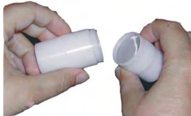
5. Insert the mouthpiece in the handle. The mouthpiece can only be inserted in one direction. A moulded lip in the mouthpiece prevents incorrect insertion. The sensor is now ready for the next patient.
