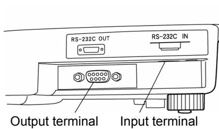
· Input terminal DIN 8-pin (Pin No.1 is not used.)
