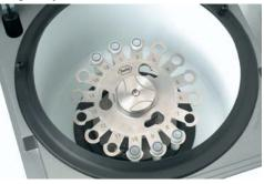
Figure 7: MagNA Lyser Removable Rotor
