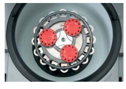
Figure 6: Retention plate in open (unsecured) position. The curved lines on the retention plate do not align with the curved marks in the center on the shaft.
