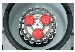
Figure 5: Retention plate in closed (secured) position. The curved lines on the retention plate align with the curved marks in the center on the shaft.
