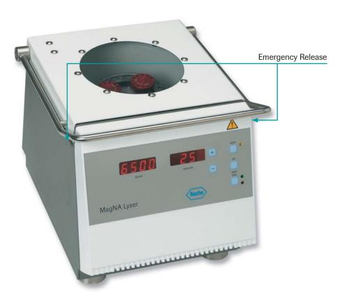
Figure 11: Emergency Interlock Override
