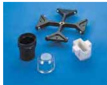
Swinging bucket rotor 75008179 with round bucket 75008172 (left), aerosol tight cap 75008173 (middle) and cyto bucket 75008176 (right)
