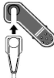
3. Slide the second Dura-Y sensor button along the other ear clip slot until the second sensor pad is fully engaged in its side of the clip.
