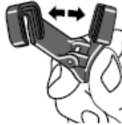
2. Slide one of the Dura-Y sensor alignment buttons along the ear clip slot until the sensor pad is fully engaged in the clip.
