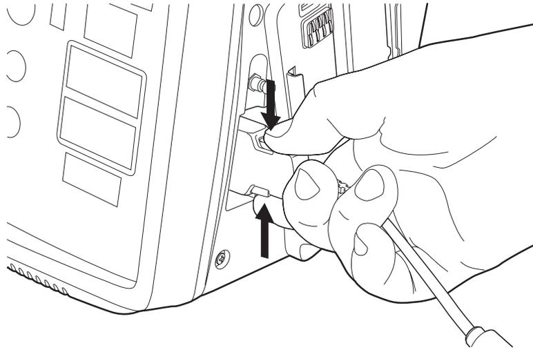
**Figure 4-13: Insert SpO<sub>2</sub> Cable into SpO<sub>2</sub> Connector**
