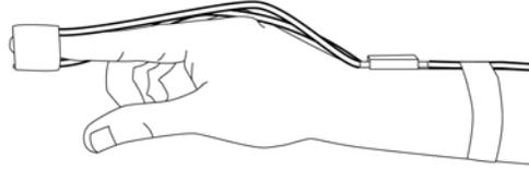
**Figure 4-7: Multi-Site Finger Placement (940SD)**
