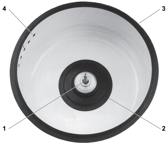
Figure 1-1. Interior View of the Spinchron DLX Centrifuge Rotor Chamber
