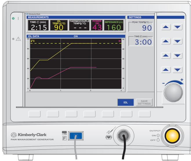
Figure 7-20 IDL MODE – ON Display (Secondary Thermocouple Disabled)
