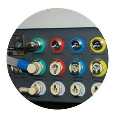
**Figure 2. Color-coded inlet connectors.** Color-coded inlets with quick connects decrease assembly time and allow the use of multiple buffers and solutions without bottle switching. The level sensors, when connected to the reservoir bottle sensors, detect if bottles are empty or full.
