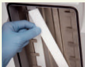
2. Insert two Humidity Control Cards into the lid and saturate with water.
