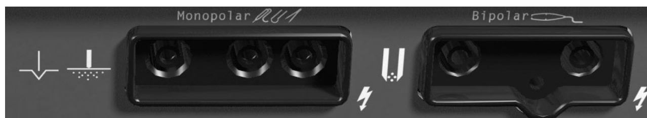
Monopolar Handswitching Receptacle Accepts standard 3-pin handpieces. Connect handswitching accessories.
