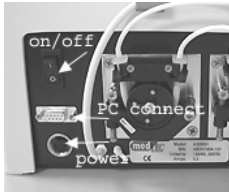
The AutoBlot uses a power supply that permits a wide range of voltages and frequencies. Although line conditioners and surge protection are not required, the instrument may be plugged into either.
