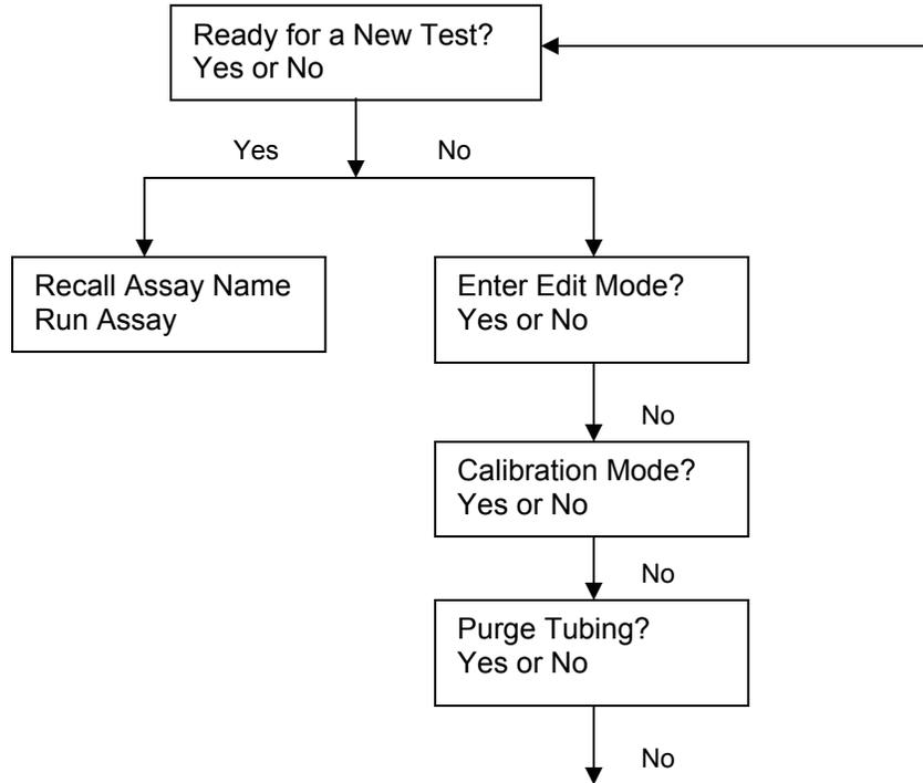
**Ready for a New Test** is the first prompt you receive when the AutoBlot is turned on. From here you can recall and run a previously programmed assay. This routine also contains the Pump Prime routine.
