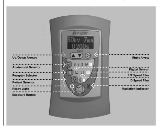
Figure 2 Preva Operator Panel
