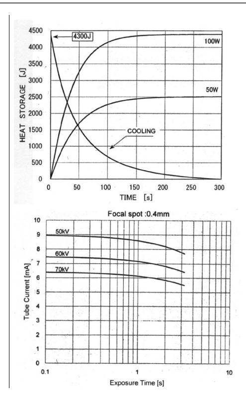
Figure 8 Toshiba Tube Rating Charts
