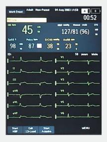
In 12-lead preview mode, 12 waves are viewable on-screen, in addition to numeric vital sign values. All waves print on the strip chart printer in 3x4 format.
