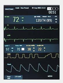
A typical *monitoring view* shows some basic patient information, the date, time and battery status. Next are the numerics and waveforms. The bottom half of the screen shows additional monitoring numerics followed by their waveforms, and *soft keys* for customizing the display, setting and responding to alarms, and scrolling through screens to view additional monitoring data.
