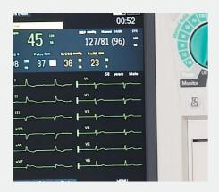
The 8.4-inch color display is well protected against damage. Recessed behind a 3-millimeter non-reflective polycarbonate shield, framed and backed in an energy-absorbing foam blanket, and supported by a rigid magnesium casting, it endures routine impact from bumps, knocks, and even drops.
