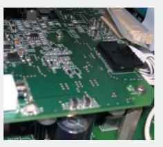
Internal assemblies are rugged. Latched connectors hold cables in place to ensure uninterrupted communications between circuit boards. And every circuit board is aggressively reinforced, braced and fastened at multiple points, keeping the device's internal structure rigid, even in high vibration environments.
