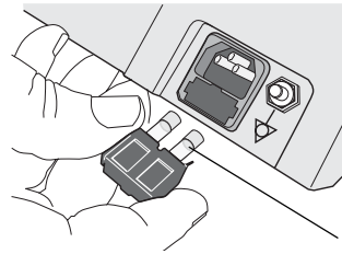
Figure 45. AC Fuses Removed
