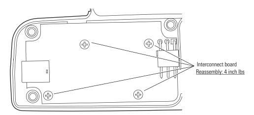
**Note** An early version of the Interconnect board included a photosensor attached by a 4-wire cable. If this photosensor and cable are present, clip the cables close to the board and remove the cable and photosensor.
