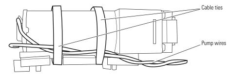
NIBP disassembly, part 3: Removing the valve assembly
