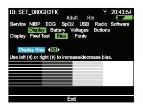
Use the controls indicated to set the bias. Bias is optimized when the visible shimmer in the test pattern is reduced to the minimum level.
