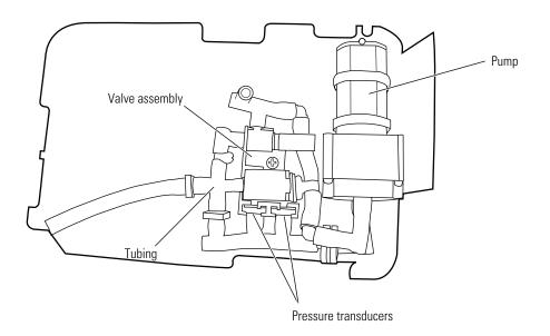
4. Disconnect the two tubing sections from the pump.
