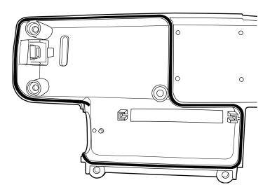
REASSEMBLY: When the rubber seal is properly installed, the ends of the seal extend into the I/O panel opening.
