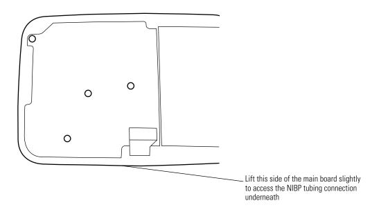
6. Disconnect the NIBP tubing from the air inlet/filter port.
