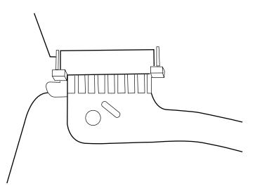
8. Disconnect the  $SpO_2$  (flex) cable from connector J3 on the back of the main board.
