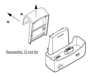
2. Slide the handle up and off of the shoulder screws.
