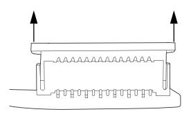
2. Insert the flex cable into the connector.
