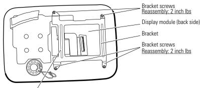
REASSEMBLY: The display module cable lies under the bracket.
