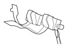
6. The connector assembly is held in place by the two snap-in clips and by an adhesive gasket. Remove the assembly by pushing in the clips while applying upward pressure on the assembly to break the grip of the gasket.
