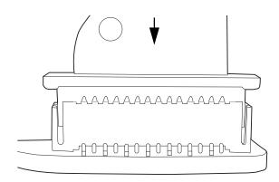
3. Slide the latching piece toward the connector body until it clicks into place.
