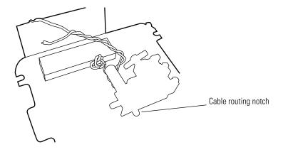
11. Remove the single screw securing the valve assembly to the main board.
