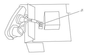
12. Disconnect the I/O panel connector from J1 on the Power board.
