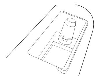
6. Remove the Power/USB flex connector assembly.
