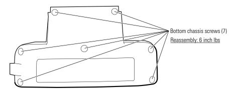
REASSEMBLY:Note the three screw holes that have nylon washers. These washers must be used in these screw holes.
