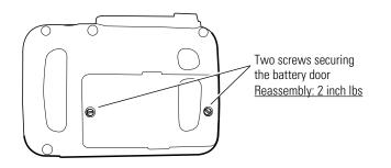
2. Remove the battery assembly from the battery compartment.
