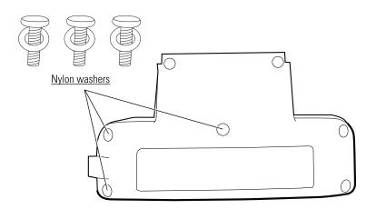
2. Remove the threadlocking screw and nylon washer from the bottom of the I/O panel.
