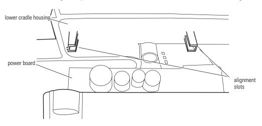
REASSEMBLY: Align the power board with the slots in the lower cradle housing.
