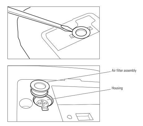
2. Remove and discard the air filter, and replace it with a new one.
