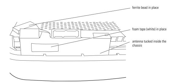
**Note** If the radio card or the antenna has been moved out of position, return the monitor to a qualified Welch Allyn service center. The radio and the antenna are not field-serviceable components.
