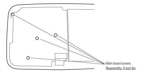
5. Lift the top of the main board slightly away from the chassis to access the NIBP tubing connection to the air inlet/filter.
