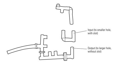
NIBP disassembly, part 2: Removing the pump
