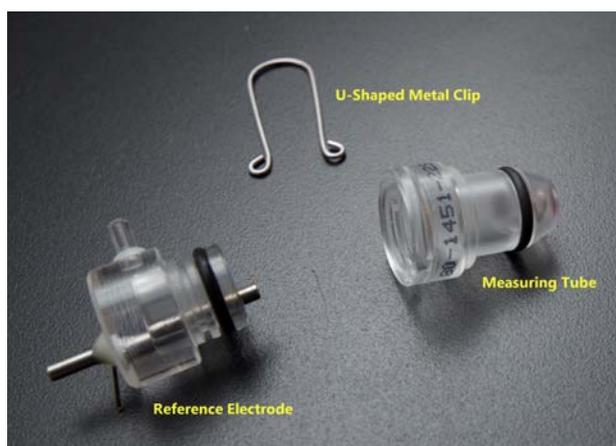
6. Place the measuring tube on a clean counter with the red or pink aperture facing up. Drop two drops of bleach onto the aperture and let it soak for ten minutes.
