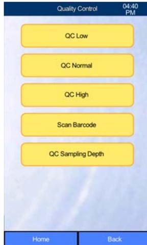
3. Select **Scan Barcode**, then scan the 2D barcode on the HM5 value assignment sheet provided with the control tube.
