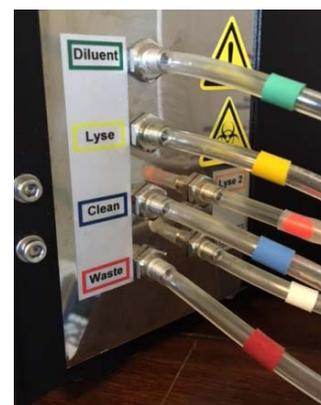
13. Attach the waste tube (red) to the top of the large white waste cap. Leave the other ends of the five reagent tubes free for now.
