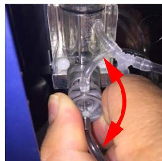
5. Disconnect the tubing and pull off the U-shaped clip so the two pieces can be separated.
