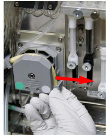
6. Slide the gray attachments toward the center of the yellow pump tube.
