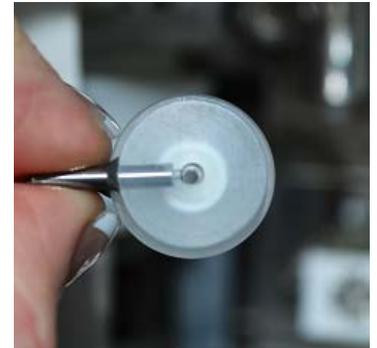
10. After it has soaked for a couple of minutes, clean the top and bottom surfaces of the Wash Head by wiping thoroughly with a moist, lint-free tissue to remove all salt residue. Large, hard salt residues may require longer soaking times.
