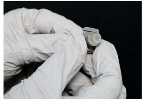
9. Slide the gray attachments down onto the clear connectors so that the connectors fit snugly into the gray pieces.
