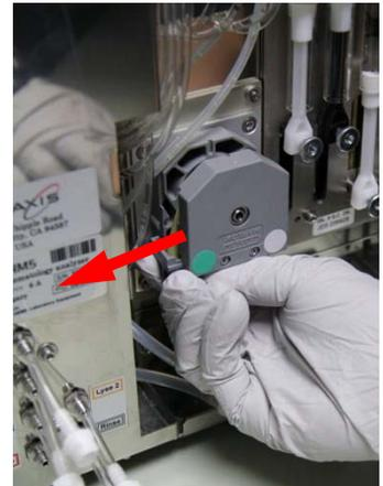
5. Grasp the bottom right tube connector (white band) and push it to the right. The connector slides out, freeing the right end of the tube.
