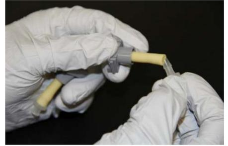
8. Place the two gray attachments onto the new pump tube. Connect either end of the new yellow pump tube to the clear connectors.
