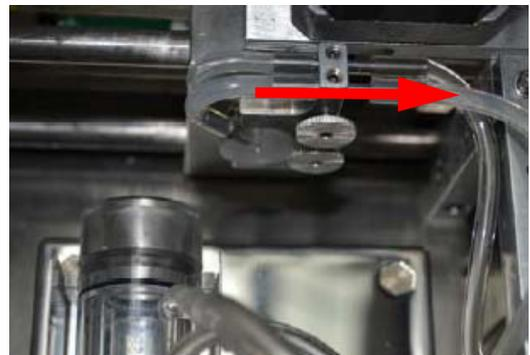
5. Loosen the thumbscrews (solid circle), and remove both completely. Take care not to drop them into the counting chamber (dashed circle).
