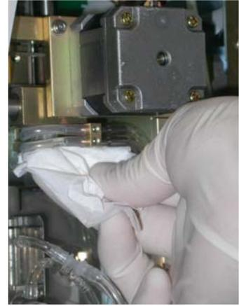
Upon removal, inspect the Wash Head for salt accumulation on the top *and* bottom surfaces.
