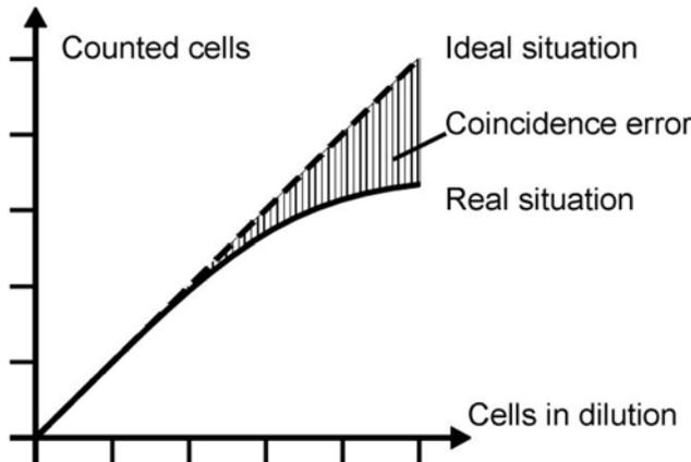
Although diluted blood is used, in cases of extremely high concentrations (such as leukemia) WBC density can be 100x higher than normal, causing two or more cells to pass through the aperture at a time, generating one pulse instead of two (or more). This is called coincidence, and results in non-linear counting of cells. Flags **m**, **M**, and **N** appear in this case.
