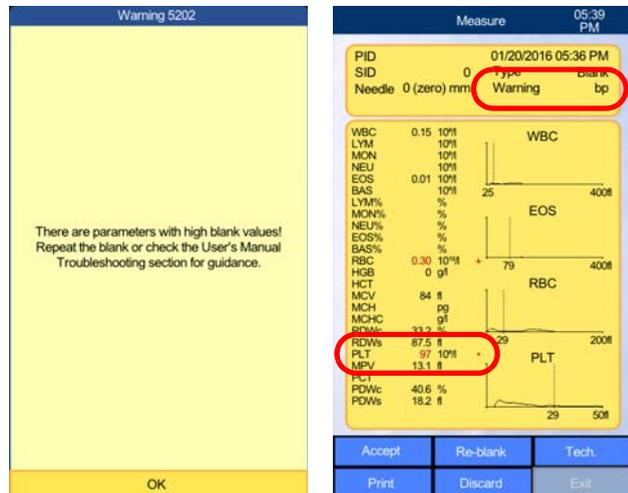
High values for the following parameters cause the blank to fail and display these warning flags:
