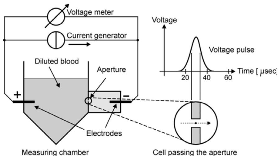
The principle of this method is that blood diluted with an isotonic solution (Diluent) conducts electric current by ionic conduction. A counting chamber made of an insulating material (plastic) holds this diluted blood, while a small circular hole (aperture) in this chamber allows the flow of diluted blood. (The analyzer aperture diameter and length is 80  $\mu\text{m}$  — the optimal size for veterinary hematology.)
