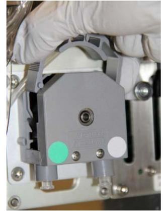
4. Grasp the bottom left tube connector (green band) and push it to the left. The connector slides out, freeing the left end of the tube.
