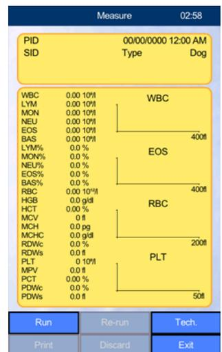
2. If the **Blank results are expired** screen appears, select **OK** to run a blank.
