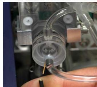
4. Grasp the measuring tube and pull while slightly twisting left and right, until it comes off. This is a push-fit part so it should pull straight out.
