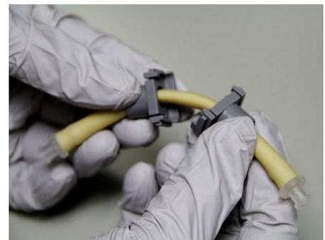
7. Disconnect the tube from the clear tube connectors.
