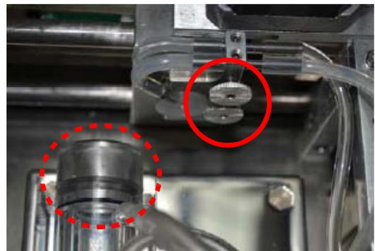
6. Gently pull the Wash Head bracket (circled) straight down, then pull the Wash Head straight down.
