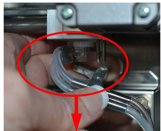
7. Remove the Wash Head from the tubing, and submerge it in a container of warm distilled water.
