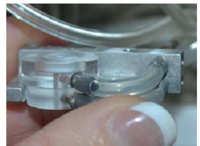
15. Align the Wash Head with the needle, and the bracket with the two thumbscrew posts, as shown at right.
