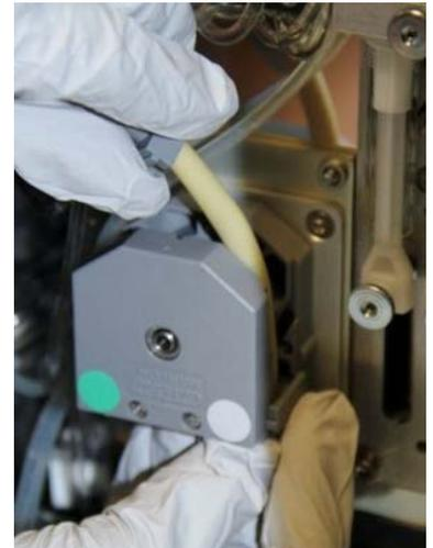
11. Reconnect the appropriate color tubes to the bottom of the pump.
