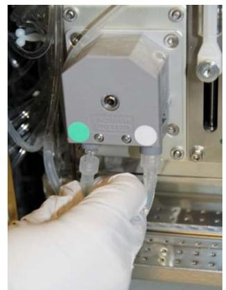
3. Use your thumb and forefinger to grasp the middle of the serrated band, then squeeze and lift the band straight up.
