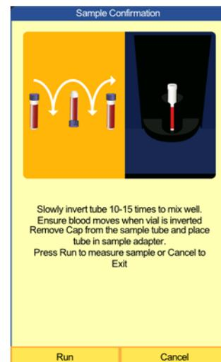
The sample is taken into the HM5 and analysis begins. The CBC process takes approximately 4 minutes for a five-part differential, and 3 minutes for a three-part differential.
