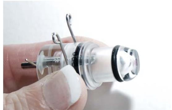
9. Push the probe back into the body of the dilution chamber and reattach tubing.
