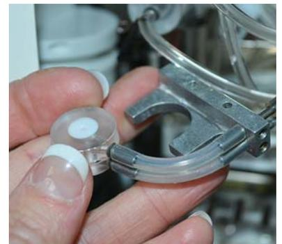
14. Slide the bottom of the Wash Head into the crescent-shaped notch, as shown.
