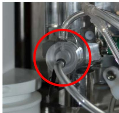
3. Disconnect the black wire from the left side of the measuring tube assembly by sliding it down and to the left.
