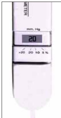
Figure 7 LCD Showing A Single IOP Measurement Of 20
