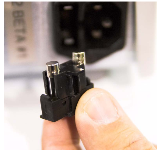
Remove fuse holder with fingers.
