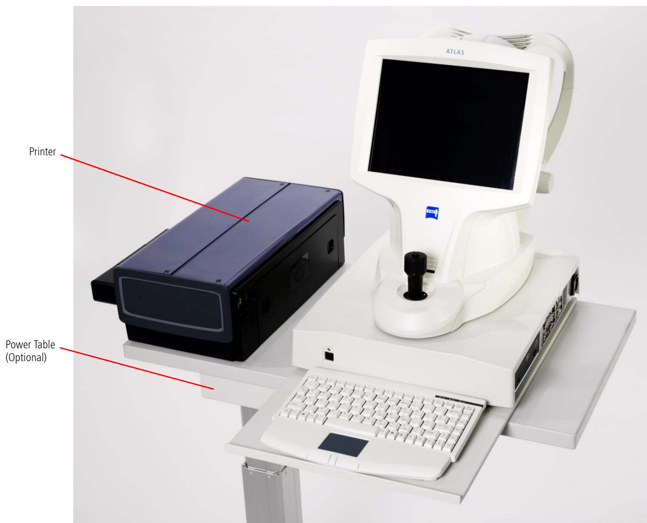
Figure 1-5 ATLAS System on Optional Power Table (with isolation transformer)
