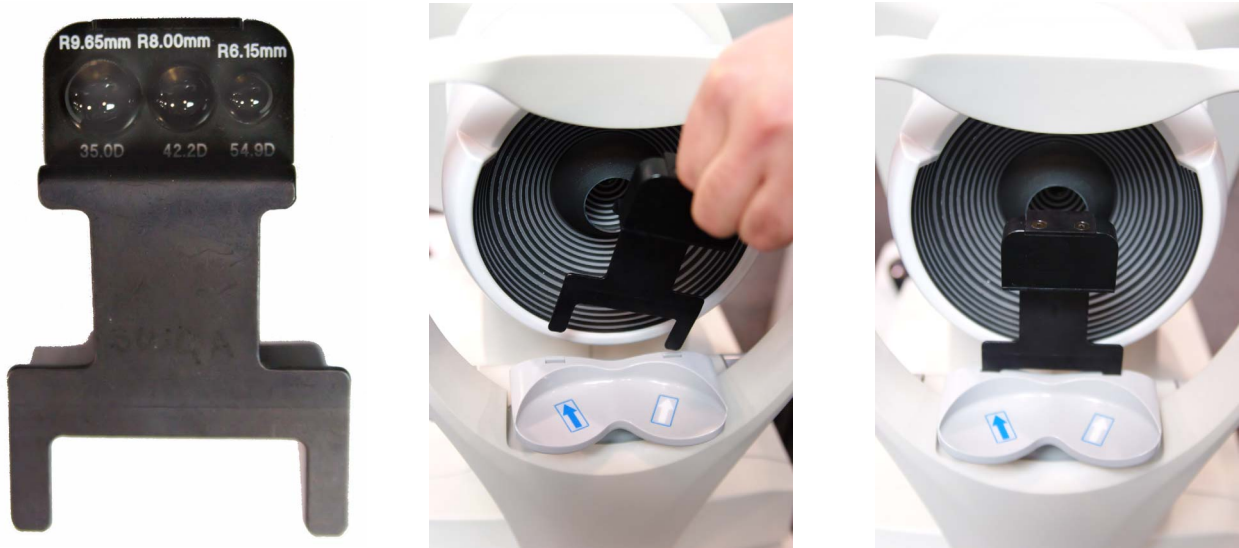
Figure H-3 Calibration Bar Inserted into Chin Rest Assembly
